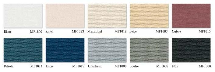
*Fiz by 3-G Mermet*—Plain weave with a soft smooth texture, this light filtering fabric is 100% fiberglass with a PVC coating and Scotchgard treatment. All 8 colors in stock. 78" roll width. Average openness 1.5%. Flame retardant: meets both NFPA 701 small- and large-scale standards.
