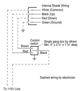
NOTE: This wiring diagram is for standard right-hand motor placement and fabric from rear of roller. For left hand motor placement with fabric from rear of roller, Red becomes "Up" and Black becomes "Down."
