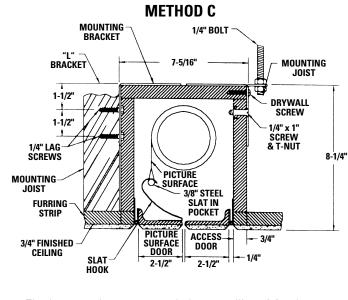
Flush mounting, recessed above ceiling. May be adapted for 1/4" paneling for ceiling and doors.
