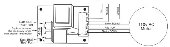
**Please Note:** When connecting data "BUS," never link an "Eye" port to another "Eye" port. You may link your BUS from "Eye" to "Aux" or "Aux" to "Aux." All BUS command input devices must connect to an "Eye" port in order to power the input device.
